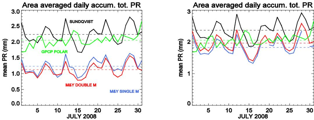
**Figure 4:** Comparison of daily total precipitations averaged over POLAR-GEM domain using SUNDQVIST (black), M&Y simple (blue) and double moment (red) with available observations (GPCP, green), with a time step of 450s (left) and 60s (right).
