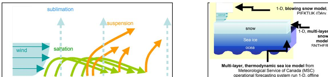
**Figure 2:** On the left: schematics of the various snow processes related to blowing snow. On the right: schematics of the three components of the NEW-RPN coupled sea ice / snow / blowing snow model.
