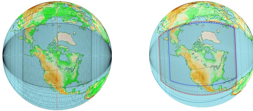
**Figure 1:** On the left: horizontal grid of the extended regional NWP model of the CMC, which became operational in the spring of 2009. On the right: the red line indicates the domain of the limited-area model that is expected to replace the CMC regional model, possibly in 2010.
