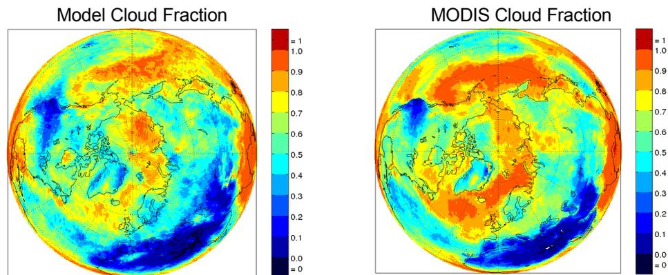
**Figure 5:** Comparison between cloud fraction fields over the Arctic averaged over July 2008: (left) generated by the CO<sub>2</sub>-slicing method, and (right) data from the MODIS satellite science team.
