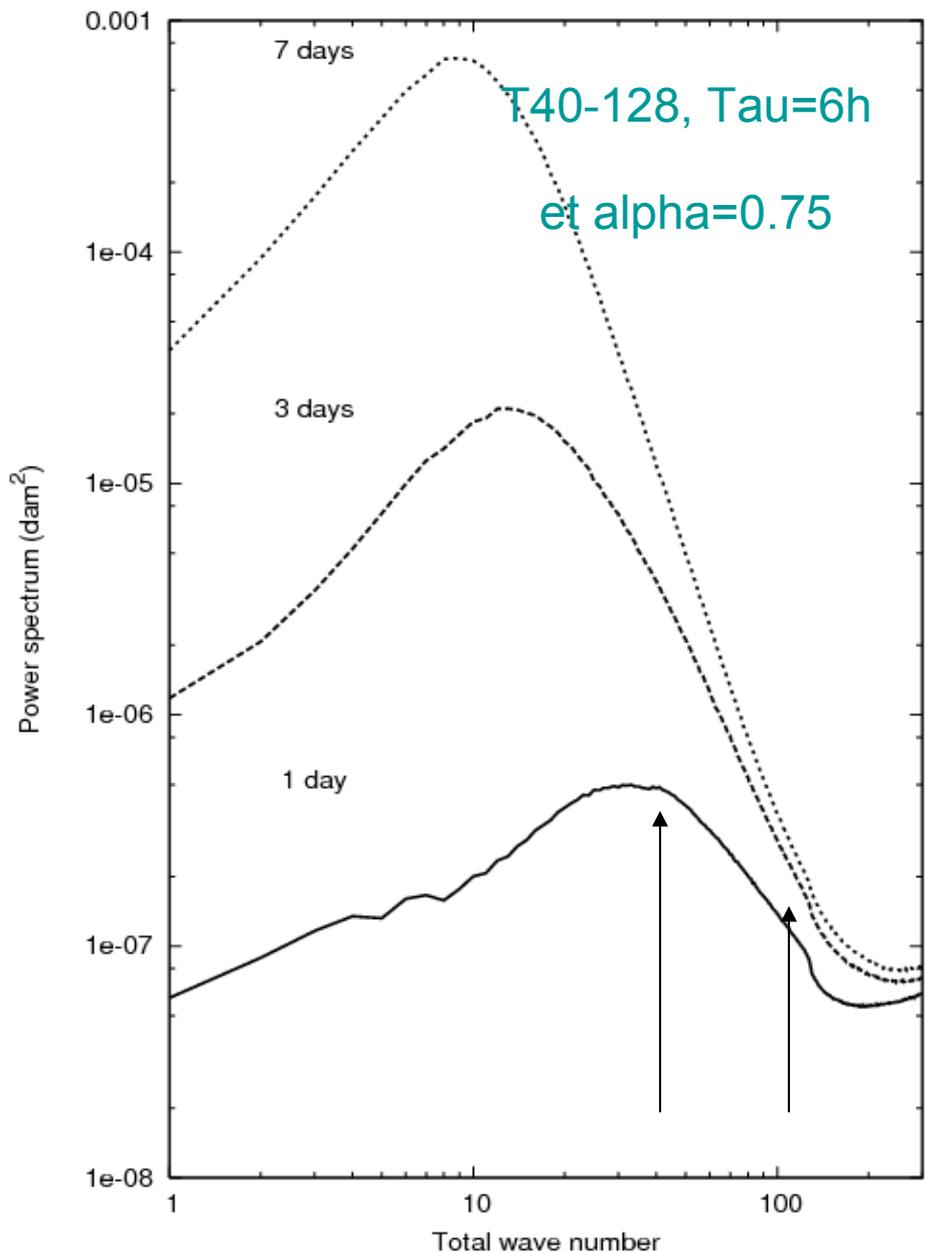
Diff. power spectrum: Z500 (with KE forcing)-(without KE forcing)
