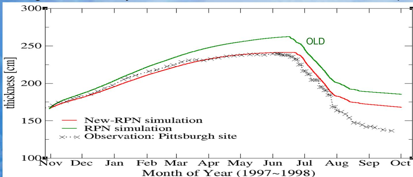
Fig. Evaluation of ice thickness [cm] for RPN and NEW-RPN and for measurements
