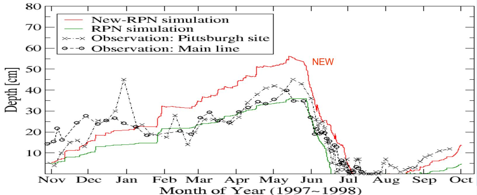
Fig. Evaluation of snow depth [cm] for RPN and NEW-RPN and for two sets of measurements.
